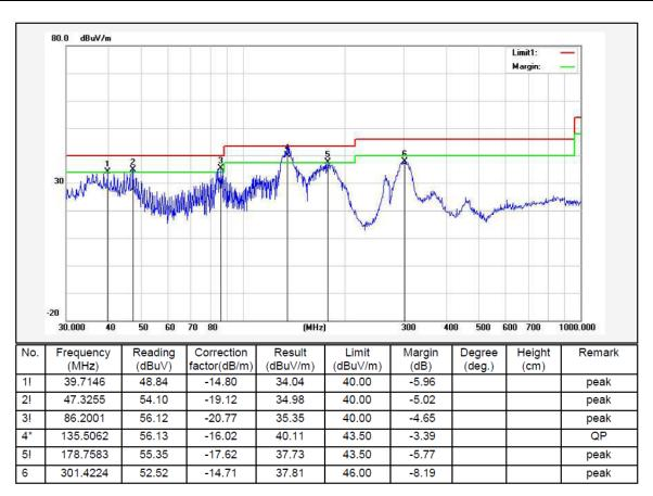
Remark: 1. Result = Reading Level + Factor, Margin = Result – Limit Factor = Ant. Factor + Cable Loss – Pre-amplifier
