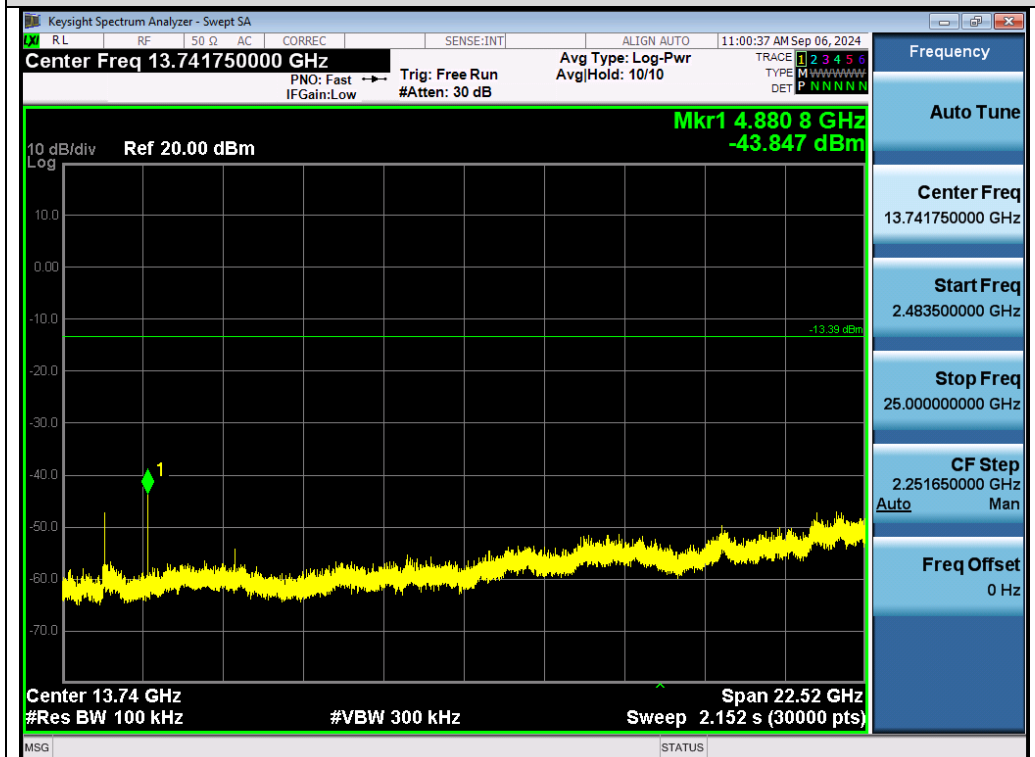
Test_Graph_LE1M_ANT1_2440_1Mbps_Higher Band Emissions
