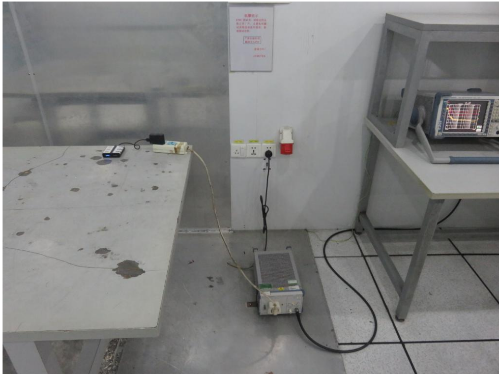
Photo of Conducted Emission Test
