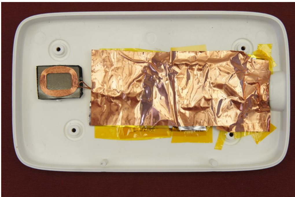
Picture 2: Power transmitter – Open, bottom side, with additional modification copper foil
