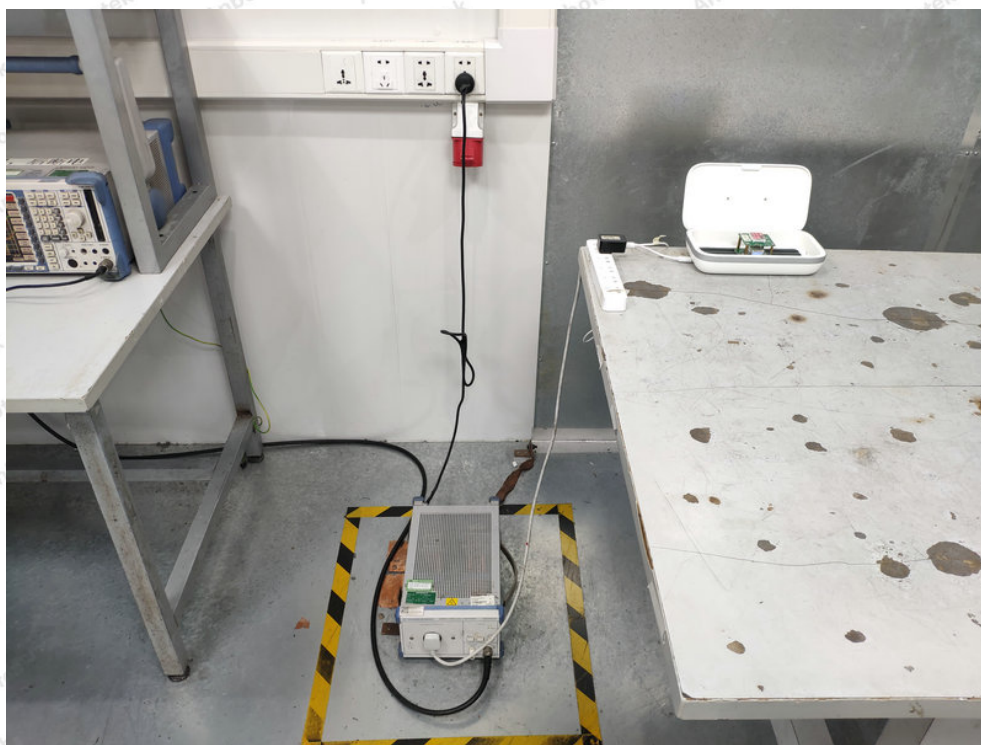
Photo of Conducted Emission Measurement
