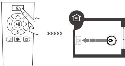
To return the robot to the charging base for recharge, press
