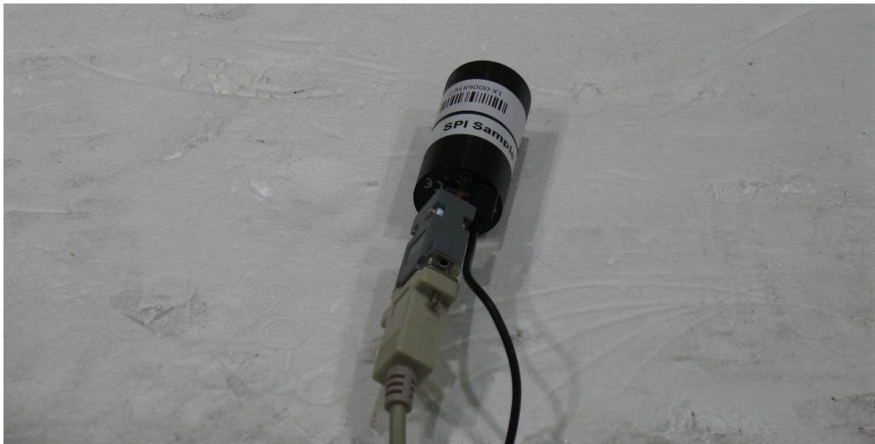
Note: Sample shown has additional SPI connector for testing purposes and is not included in normal configuration
