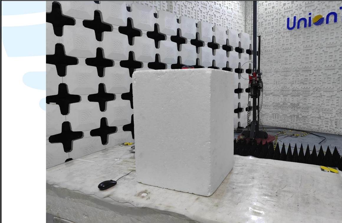
Radiated emission Test Setup (Above 1 GHz)
