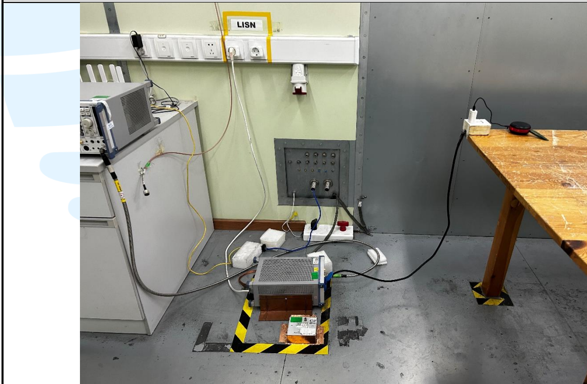
Conducted Emission Test Setup
