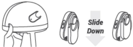
When attaching mount onto the helmet, make sure there is no dust or contaminants on the tape. Mount will not work well with the stuff on it and loosened mount can cause the entire device fall and break.
