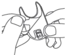
**Step 1** | Pick the right mount for the helmet, Remove the backing paper from the mount.
