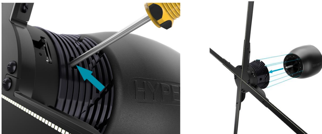
Picture 41. Unscrewing the binding screw and removing the rotor from the shaft
