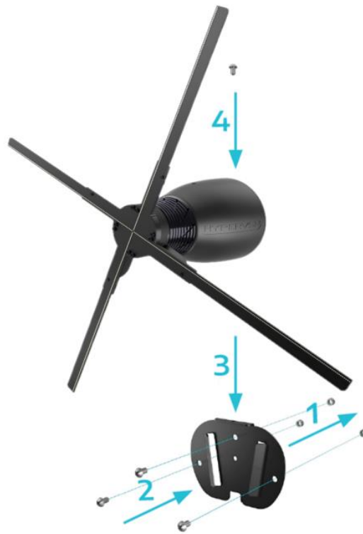
Picture 8. Device installation on a wall
