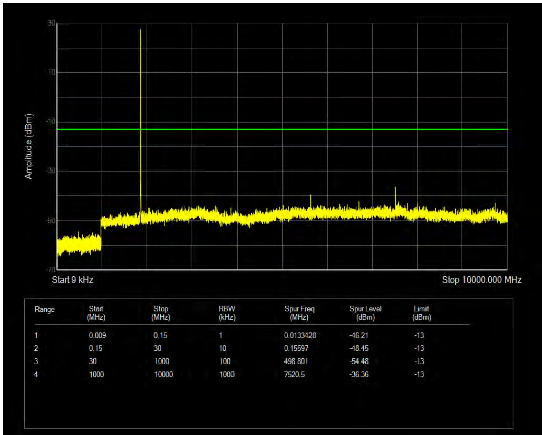
Band2 QAM16 BW=1.4MHz Channel=18900 RB Size=1 Position=#0
