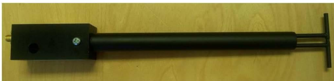
Figure 1 – MVG COMOSAR Validation Dipole
