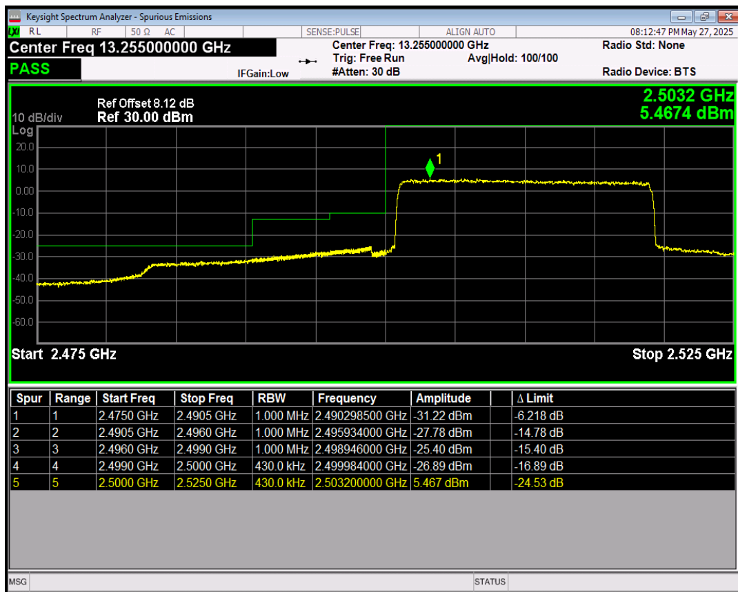
Band7 QPSK BW=20MHz Channel=20850 RB Size=1 Position=#0
