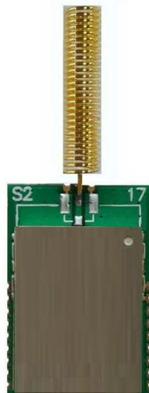
Note: The length of antenna is different for modules with different frequency
