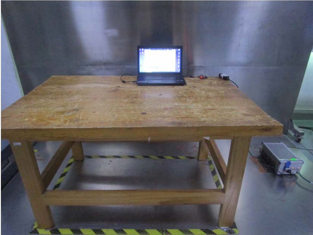
Conducted Emissions Side View
