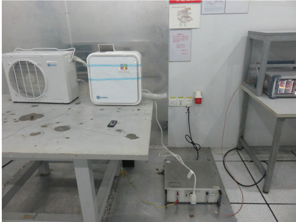
Photo of Conducted Emission Measurement
