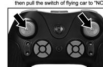
4 Place the flying car on a level surface, push the left joystick to the lower right corner, then push the right joystick to the lower right corner for 2 to 3 seconds, the indicator light of the flying car would become flashing quickly from normally on. Then it would become normally on again for another 2 to 3 seconds, that means the
