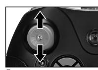
3 Place the flying car on a level surface, push the throttle joystick to the highest point and then pull back to the lowest point when the indicator light of the flying car becomes slowly flashing from guickly flashing. Then the indicator light of flying car would becomes normally on from slowly flashing.
