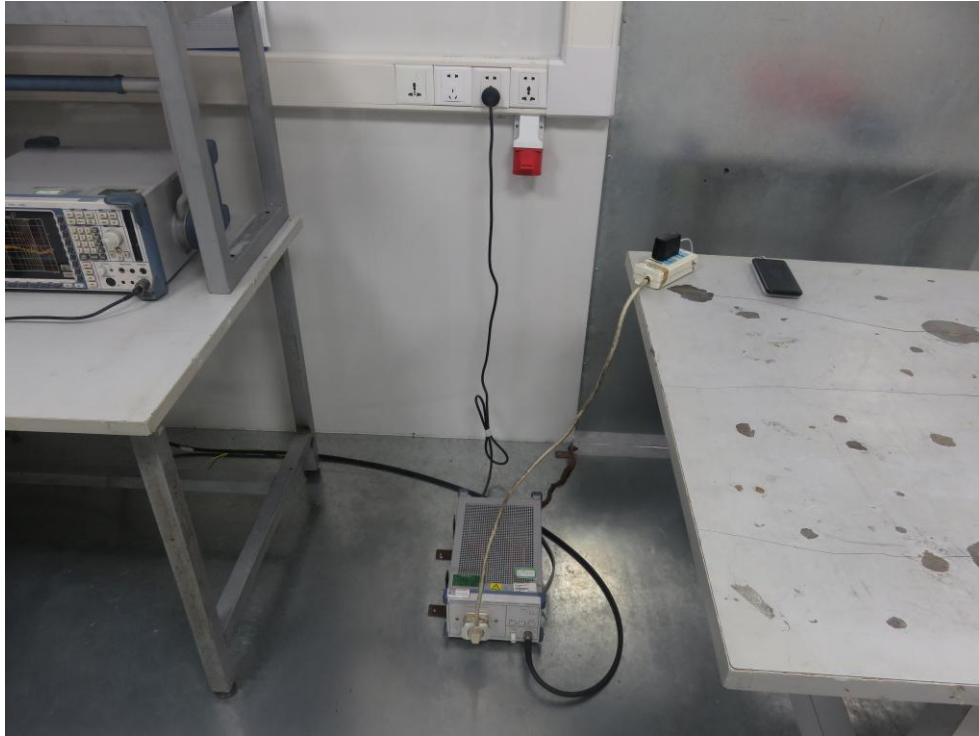
Photo of Conducted Emission Measurement
