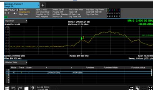
Out Of Band Emission BLE 2M_Channel 0
