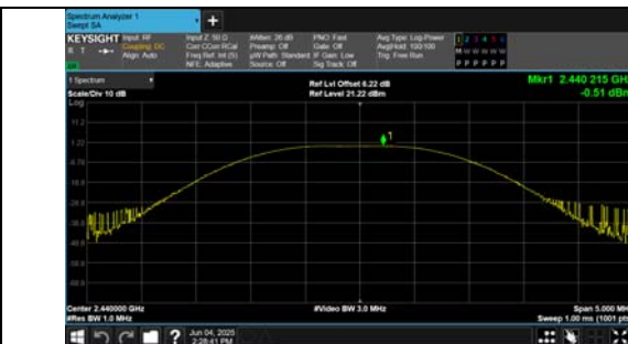
Peak Output Power BLE 1M_Channel 19
