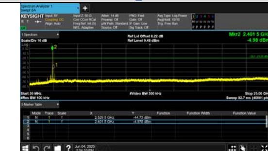
30.0 MHz - 25000.0 MHz BLE 1M_Channel 0
