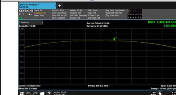
Peak Output Power BLE 2M_Channel 0
