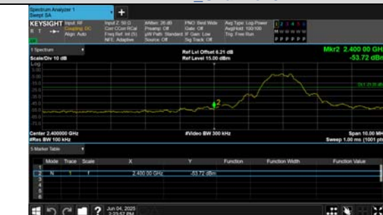
Out Of Band Emission BLE 1M_Channel 0
