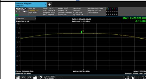
Peak Output Power BLE 2M_Channel 39
