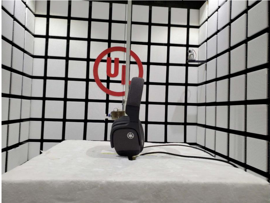
RADIATED RF MEASUREMENT SETUP (30MHz~1GHz)
