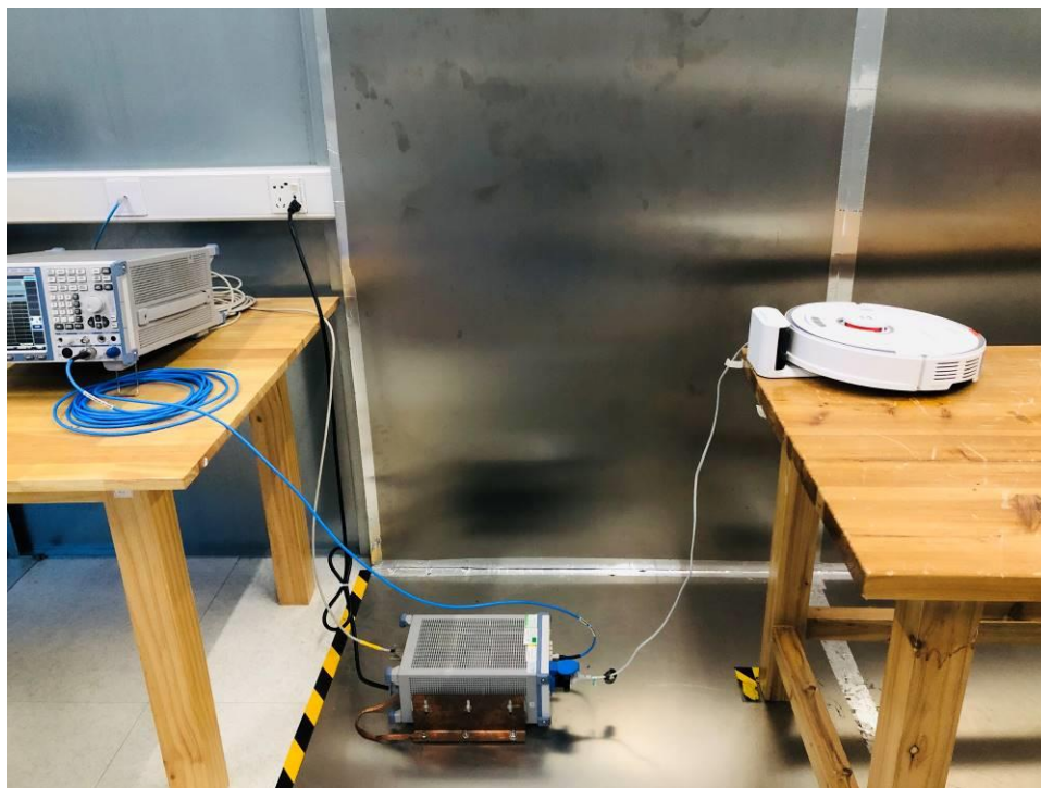
Photograph 3: Set-up photo for Conducted Emission
