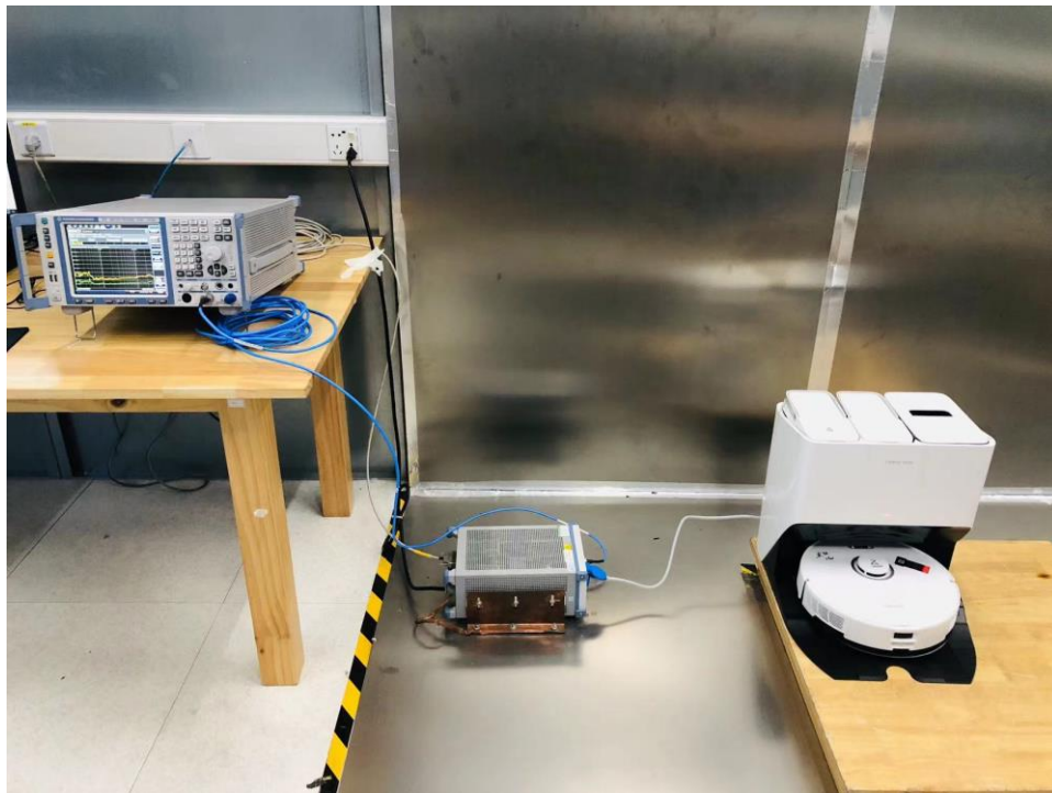
Photograph 3: Set-up photo for Conducted Emission
