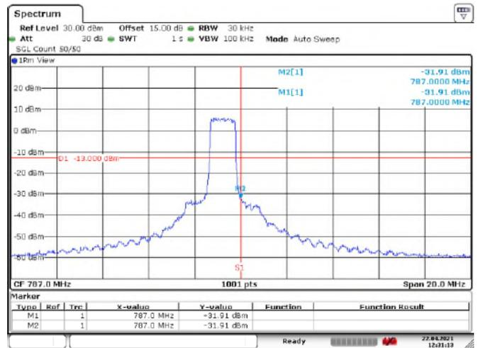
LTE Band 13\_16QAM\_Channel Bandwidth: 5 MHz
