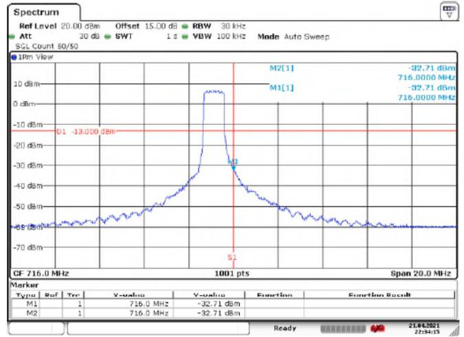
LTE Band 12\_QPSK\_Channel Bandwidth: 10 MHz
