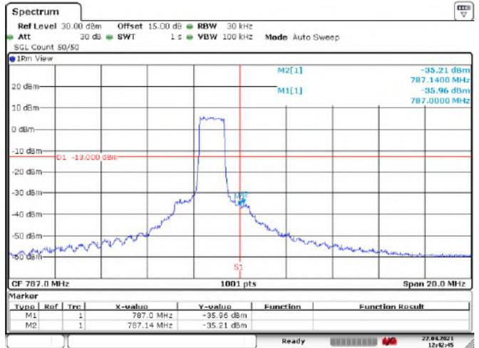
LTE Band 13\_16QAM\_Channel Bandwidth: 10 MHz
