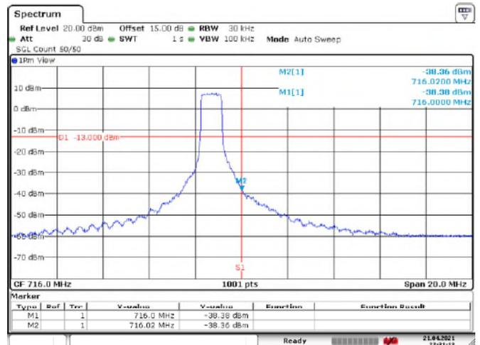
LTE Band 13\_QPSK\_Channel Bandwidth: 5 MHz
