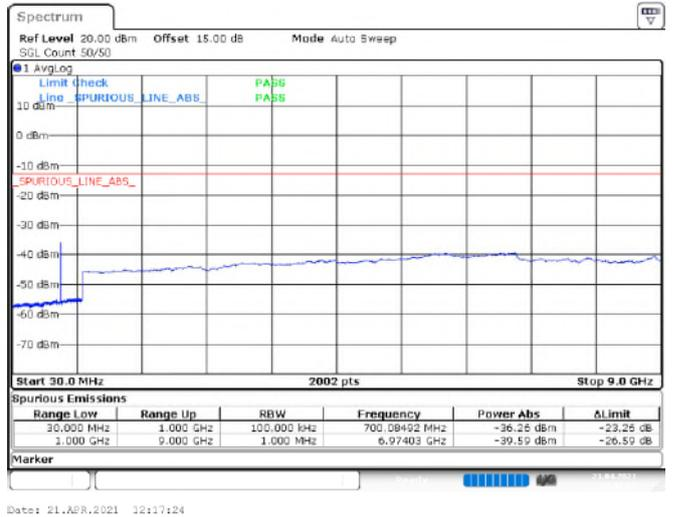
LTE Band 12\_QPSK\_Channel Bandwidth 10 MHz
