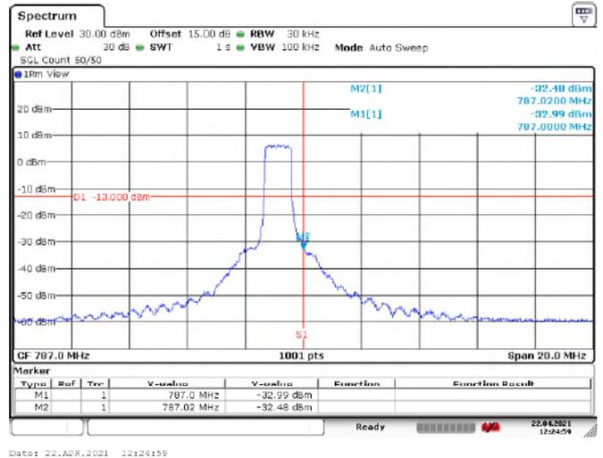
LTE Band 13\_QPSK\_Channel Bandwidth: 10 MHz
