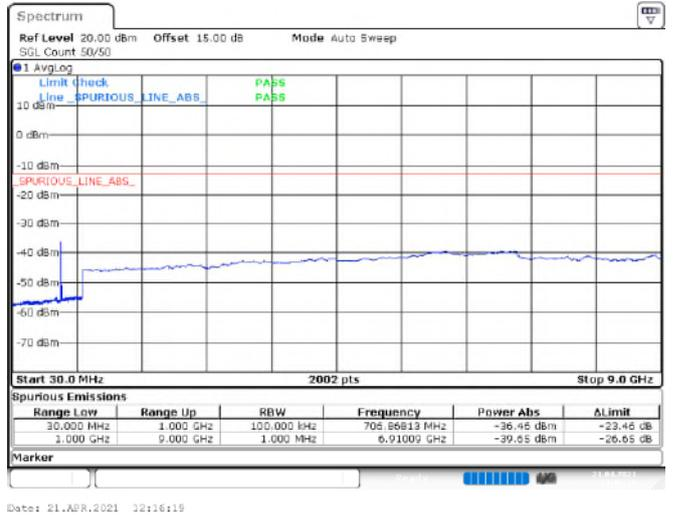
LTE Band 12\_16QAM\_Channel Bandwidth 10 MHz
