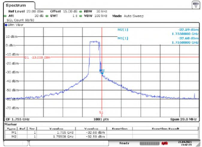
LTE Band 4\_QPSK\_Channel Bandwidth: 3 MHz
