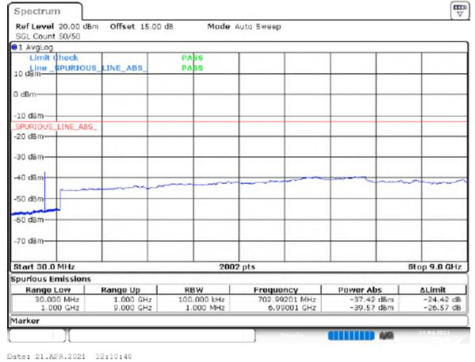
LTE Band 12\_16QAM\_Channel Bandwidth 10 MHz
