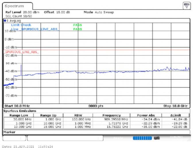
LTE Band 4\_QPSK\_Channel Bandwidth 20 MHz
