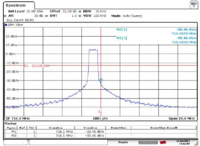
LTE Band 12\_QPSK\_Channel Bandwidth: 3 MHz
