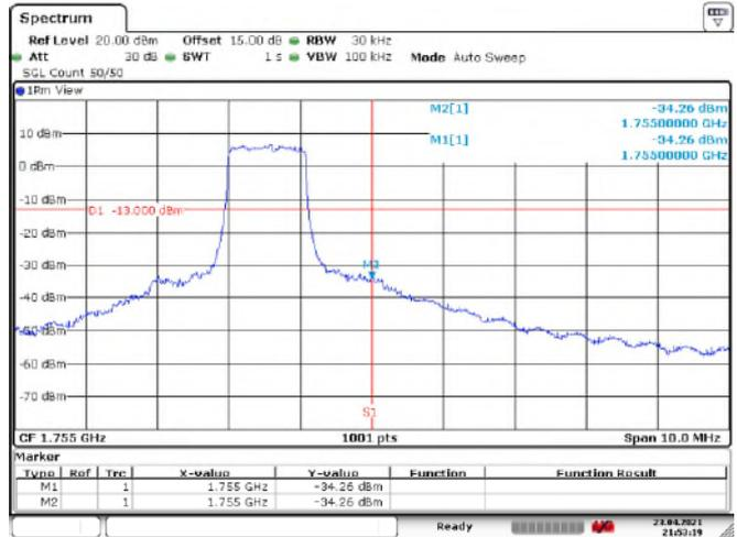
LTE Band 4\_16QAM\_Channel Bandwidth: 15 MHz
