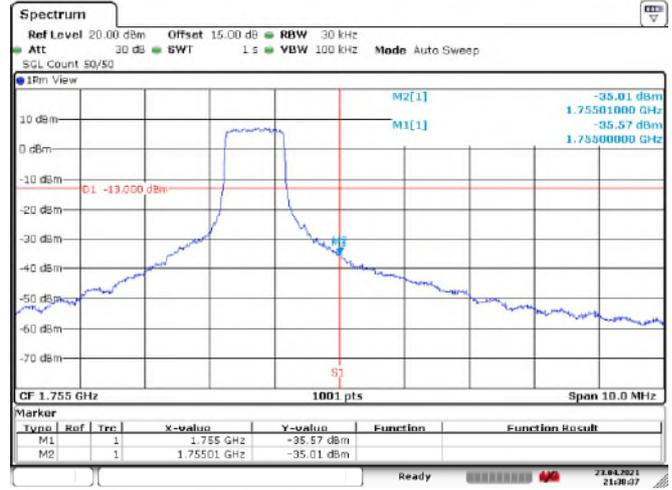
LTE Band 4\_QPSK\_Channel Bandwidth: 15 MHz
