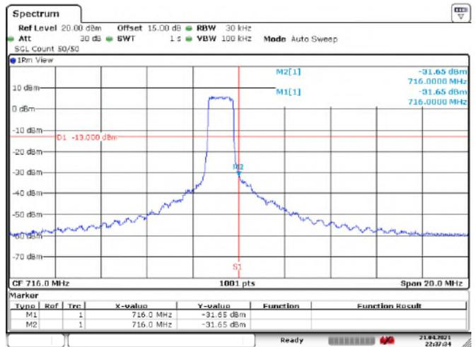
LTE Band 12\_16QAM\_Channel Bandwidth: 5 MHz
