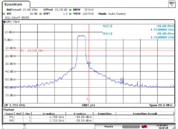
LTE Band 4\_QPSK\_Channel Bandwidth: 10 MHz
