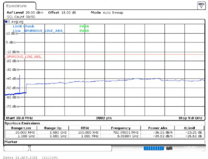
LTE Band 12\_QPSK\_Channel Bandwidth 10 MHz
