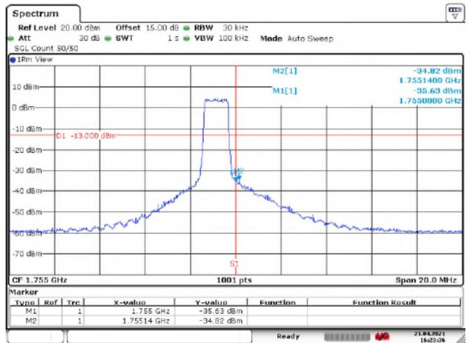
LTE Band 4\_16QAM\_Channel Bandwidth: 3 MHz
