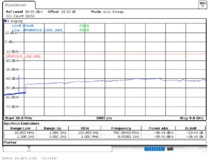
LTE Band 12\_16QAM\_Channel Bandwidth 10 MHz
