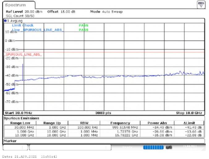
LTE Band 4\_16QAM\_Channel Bandwidth 20 MHz
