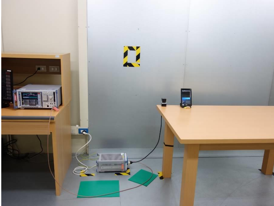
Photograph 10: Test Setup for Mains Conducted Emissions (Front View)
