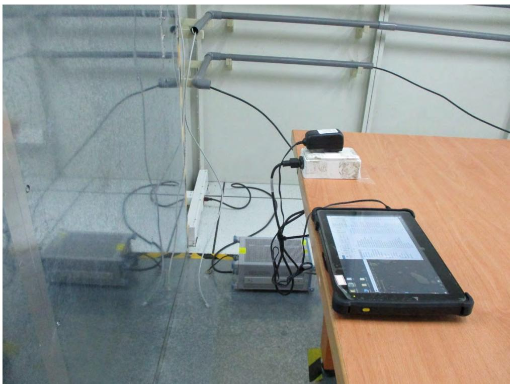
**AC Line Conducted Emissions (Mode: Charge + Transmitting with White cradle)**
