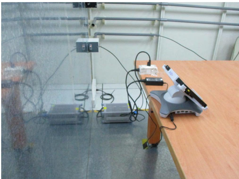
**AC Line Conducted Emissions (Mode: Charge + Transmitting with Black cradle)**
