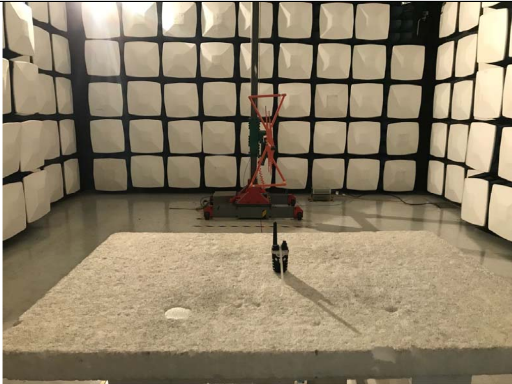
Radiated emission Test Setup (30 MHz~1 GHz)
