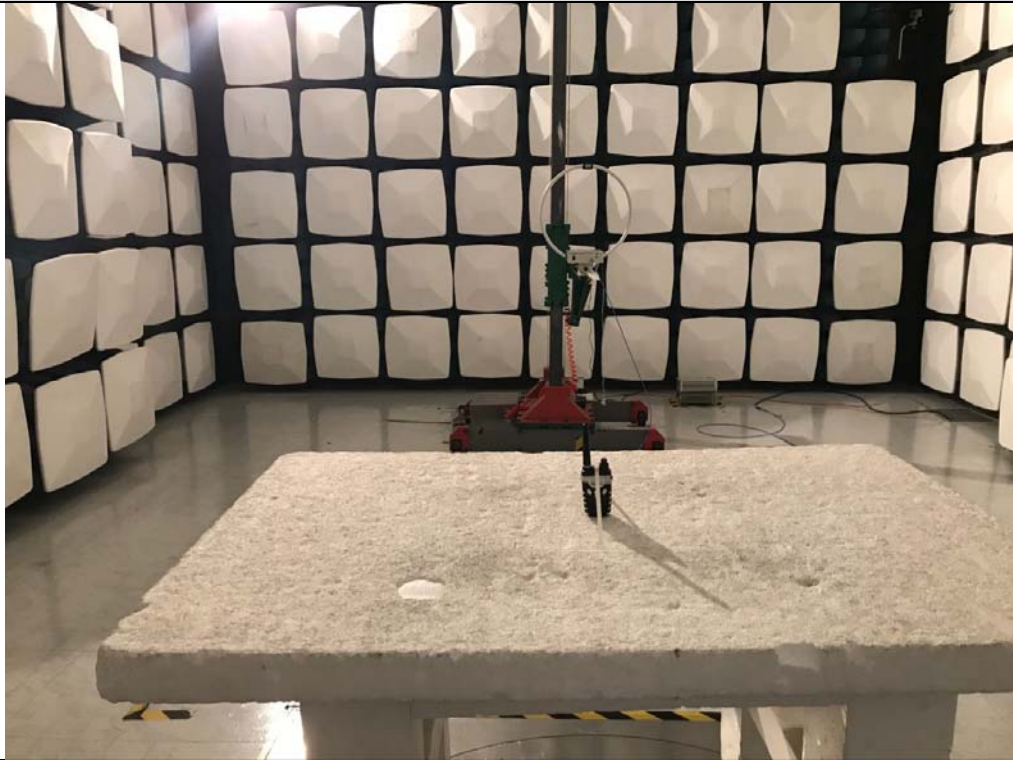
Radiated emission Test Setup (Below 30 MHz)
