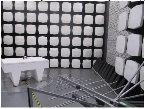
1.2 Radiated Emissions(9kHz-30MHz) Test Setup
