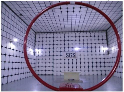
1.3 Radiated Emissions(30MHz-1GHz) Test Setup
