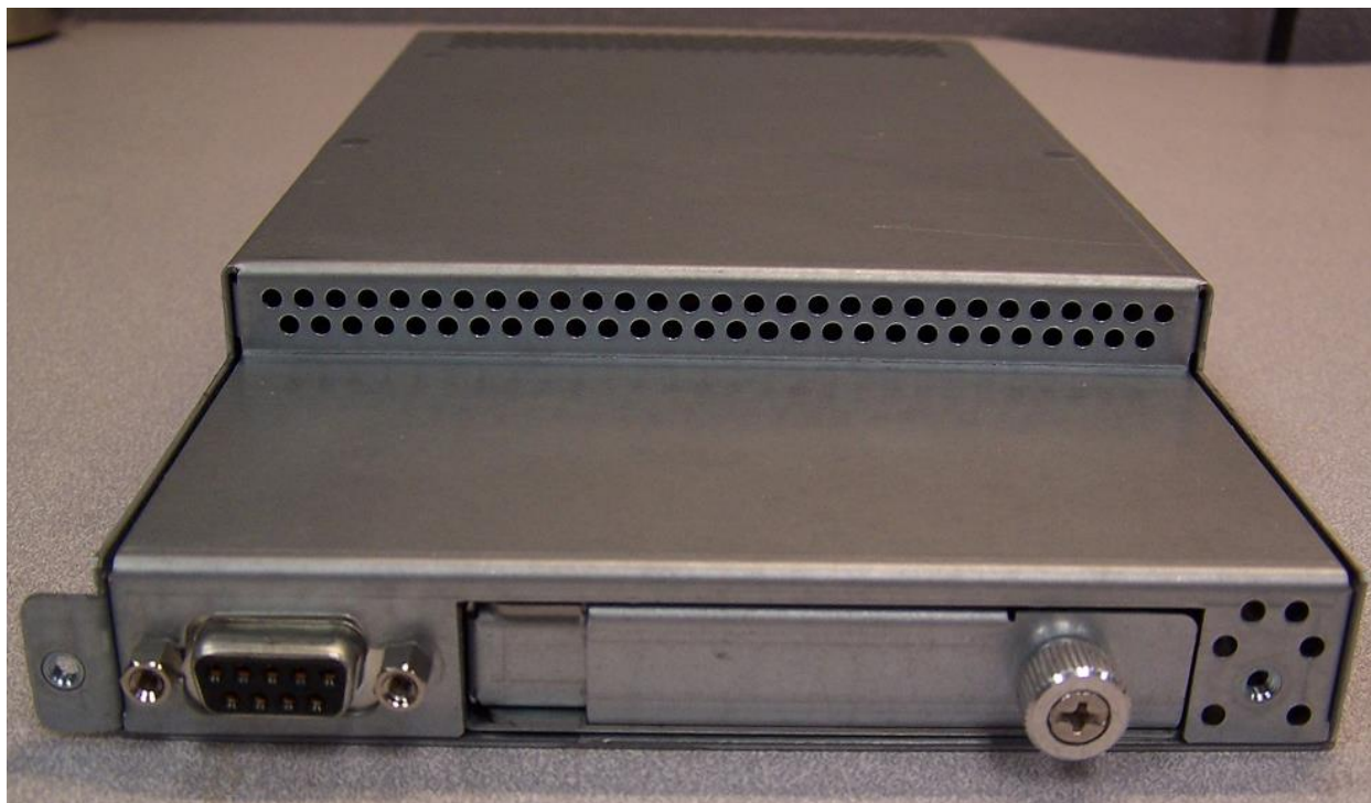
WiSP Enclosure Front with Control Cable 9-pin D-Subminiature Connector and Removable Solid State Drive Bay
