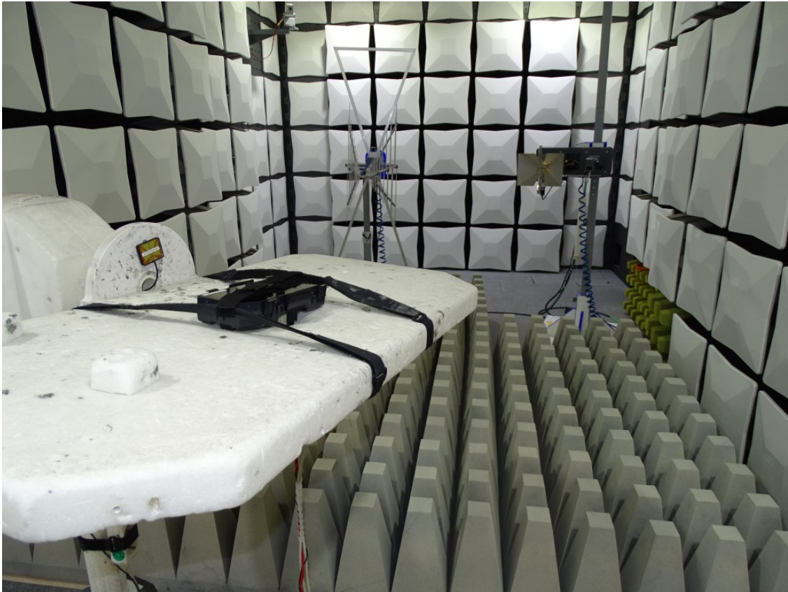
Photo 2: Test setup for radiated measurements (stand alone, EUT supplied by a battery) Above 1 GHz
