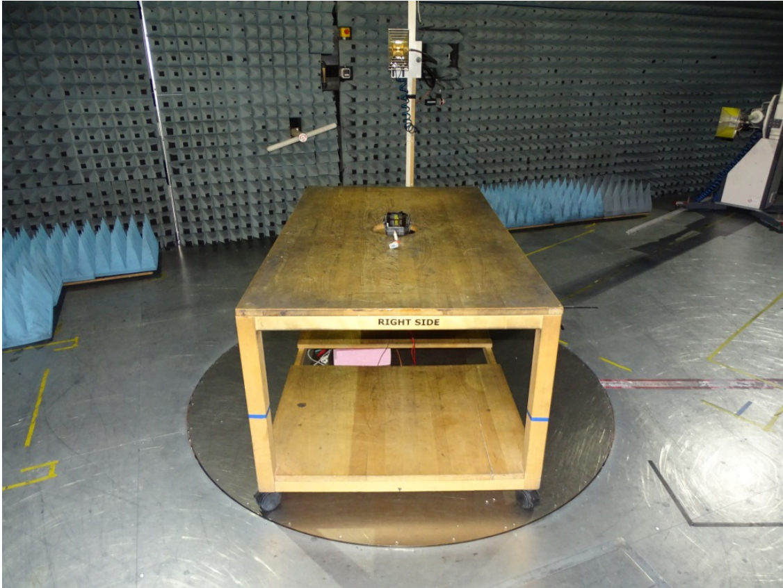
Photo 1: Test setup for radiated measurements (stand alone, EUT supplied by a battery) 30 MHz - 1 GHz
