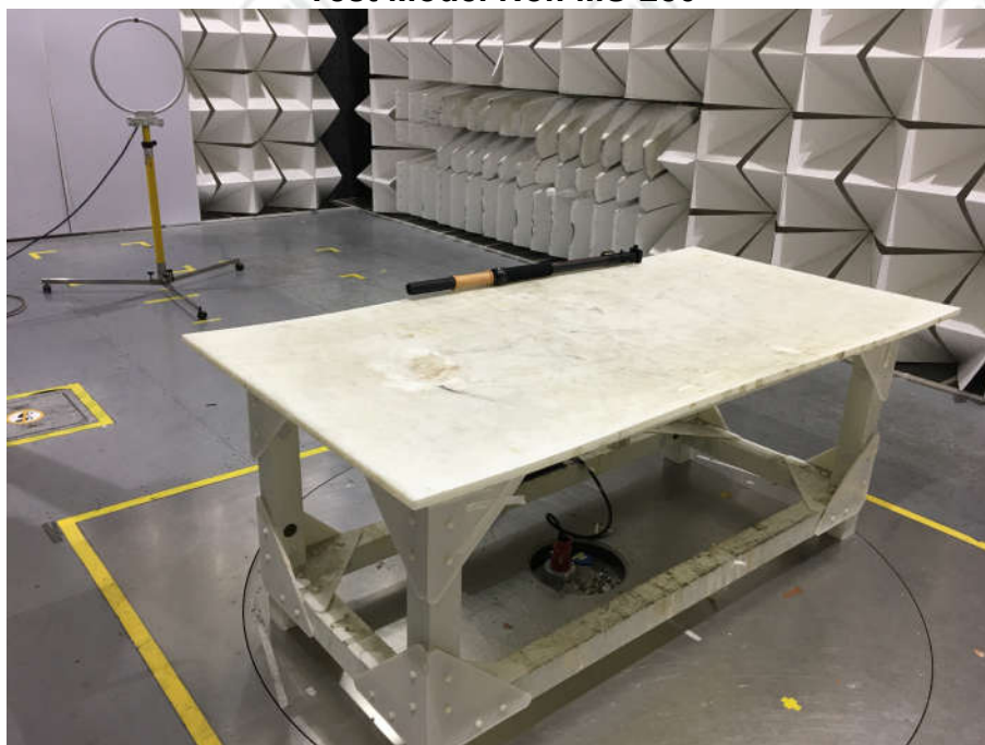
Radiated spurious emission Test Setup-1(Below 30MHz)
