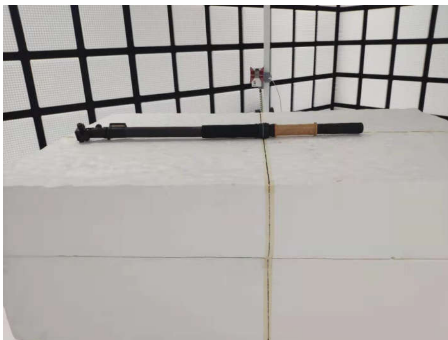
Radiated spurious emission Test Setup-3(Above 1GHz)
