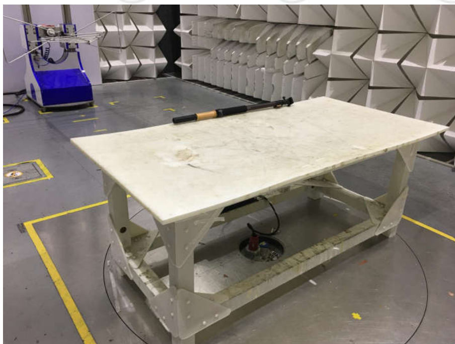
Radiated spurious emission Test Setup-2(Below 1GHz)
