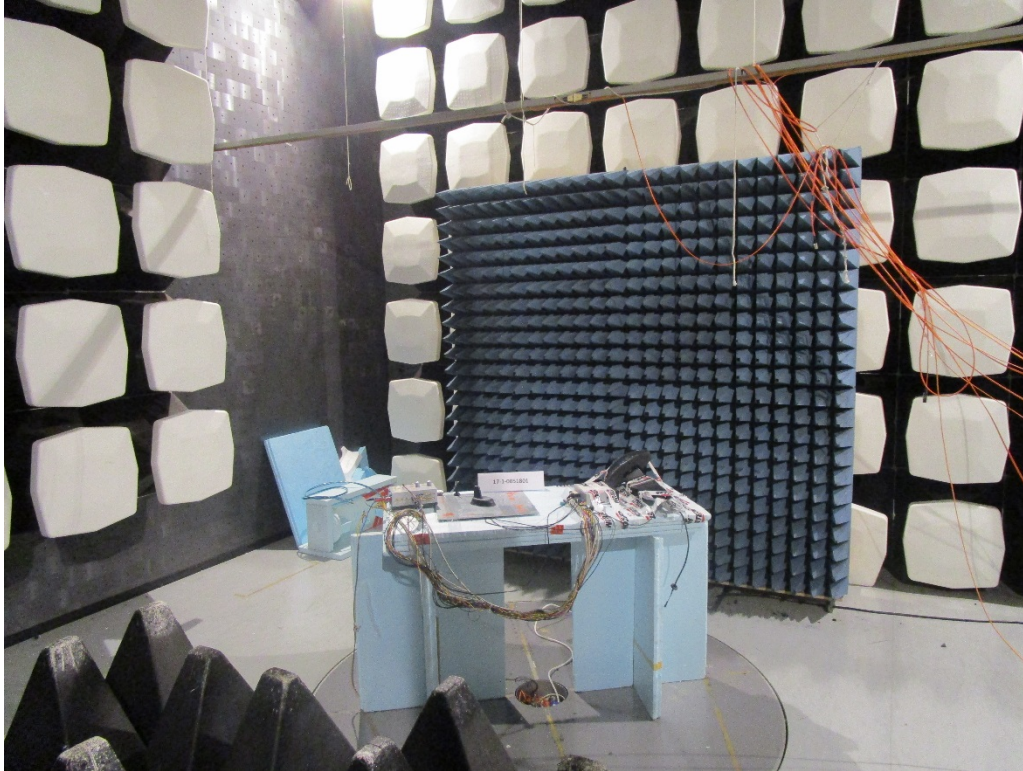
Test setup in semi anechoic room long shot view EUT laying
