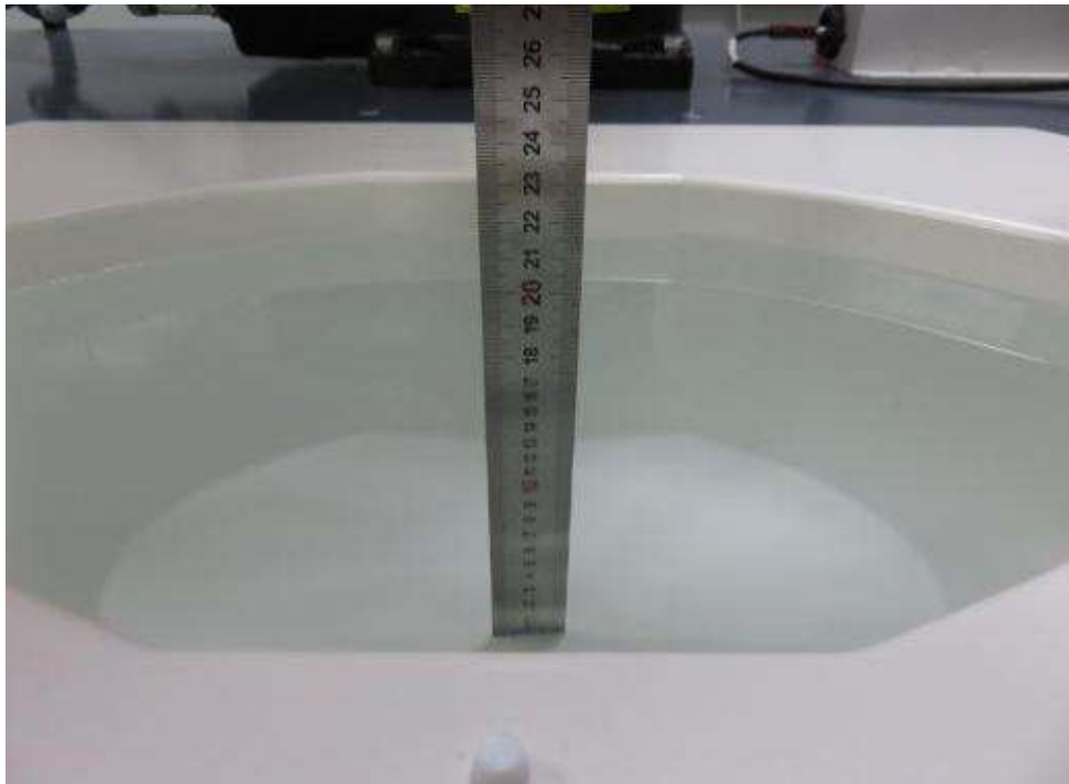
Photograph of the depth in the Body Phantom (750MHz, 16.2cm depth)
