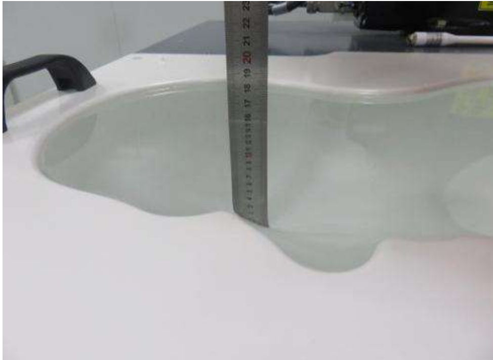
Photograph of the depth in the Head Phantom (1800MHz, 15.9cm depth)
