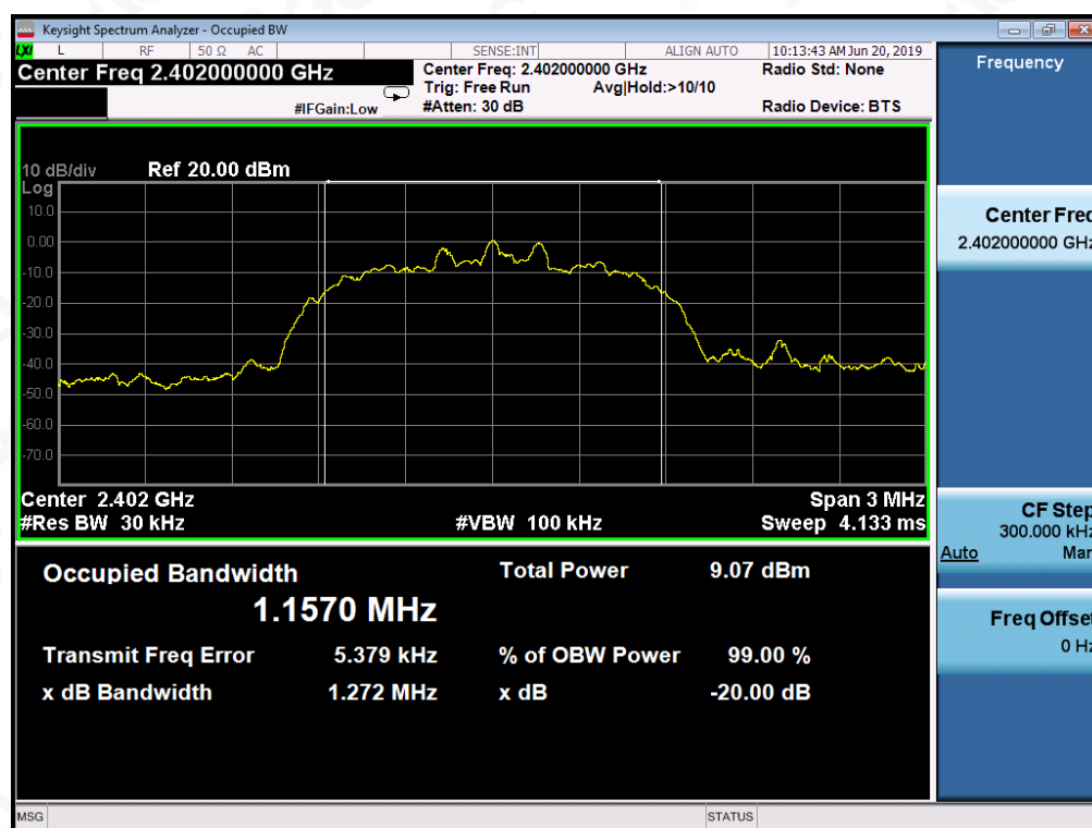
TEST PLOT OF BANDWIDTH FOR LOW CHANNEL
