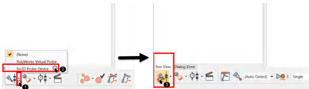
How to connect the probe in Polyworks Metrology Suite
