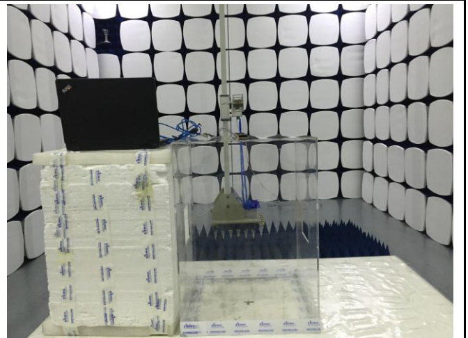
Radiated Spurious Emissions Test Setup Above 1GHz
