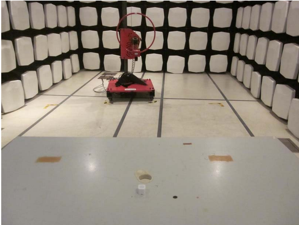
Measurement of Radiated Emission Test Set Up
