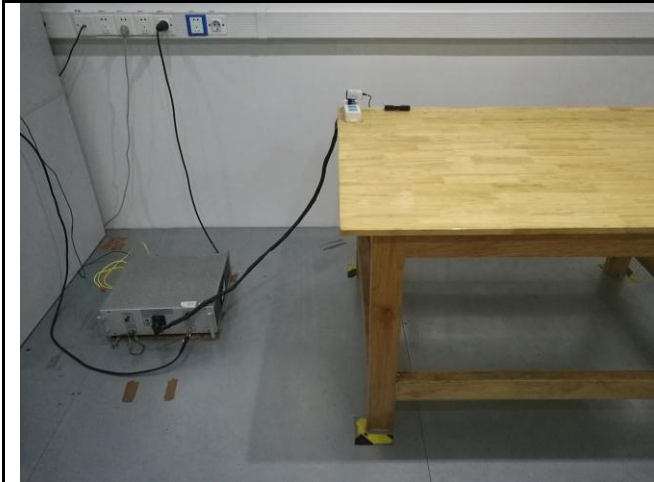
Conducted Emissions Test Setup Front View
