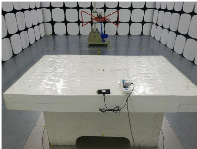
Conducted Emissions Test Setup Front View
