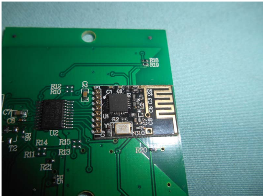
FIGURE 6 REMOTE CONTROL (M/N: WRC200T-01) CHIP AND CRYSTAL ON KEYBOARD
