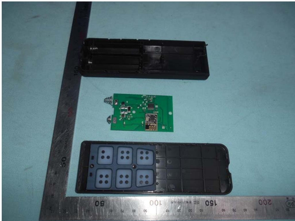
FIGURE 3 REMOTE CONTROL (M/N: WRC200T-01) COVER REMOVED IN CONTROLLER
