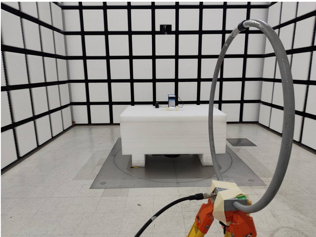
Radiated Emission Perpendicular View
