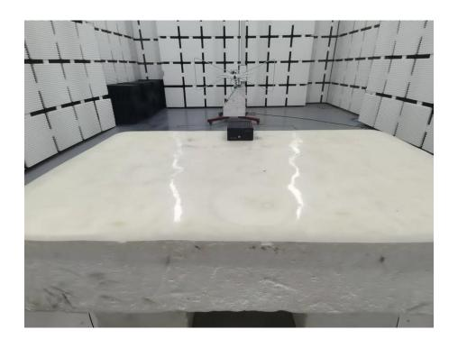
**Set-up for Radiated Spurious Emission, Above 1GHz**
