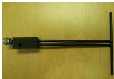
Figure 1 – MVG COMOSAR Validation Dipole
