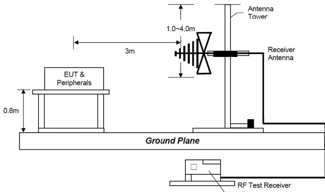
(2) Radiated Emission Test Set-Up, Frequency above 1GHz
