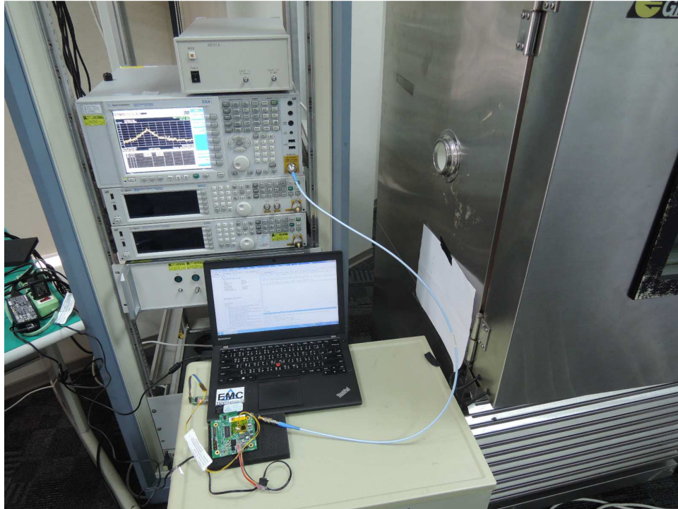
Photograph 4: Set-up for Conducted testing
