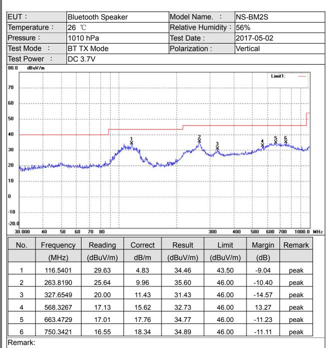
Factor = Antenna Factor + Cable Loss.
