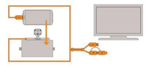
Steam VR cable: Use the usb plug with NOLO logo to connect the headset mark to PC, and the other one to connect your phone to PC.
