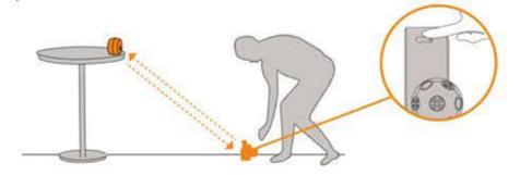
Place the headset on the ground facing the base station. Make sure there is no block between tracking sensor and base station. Press the button on the headset Marker to standardize the ground (recenter).
