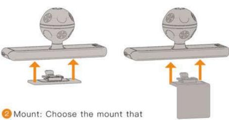
Mount: Choose the mount that fits your headset, paste it in the middle of the top of the headset with double-sided adhesive tape. Headset marker: Insert the headset marker into the mount.
