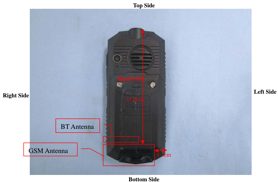
Block Diagram for EUT Antenna Position
