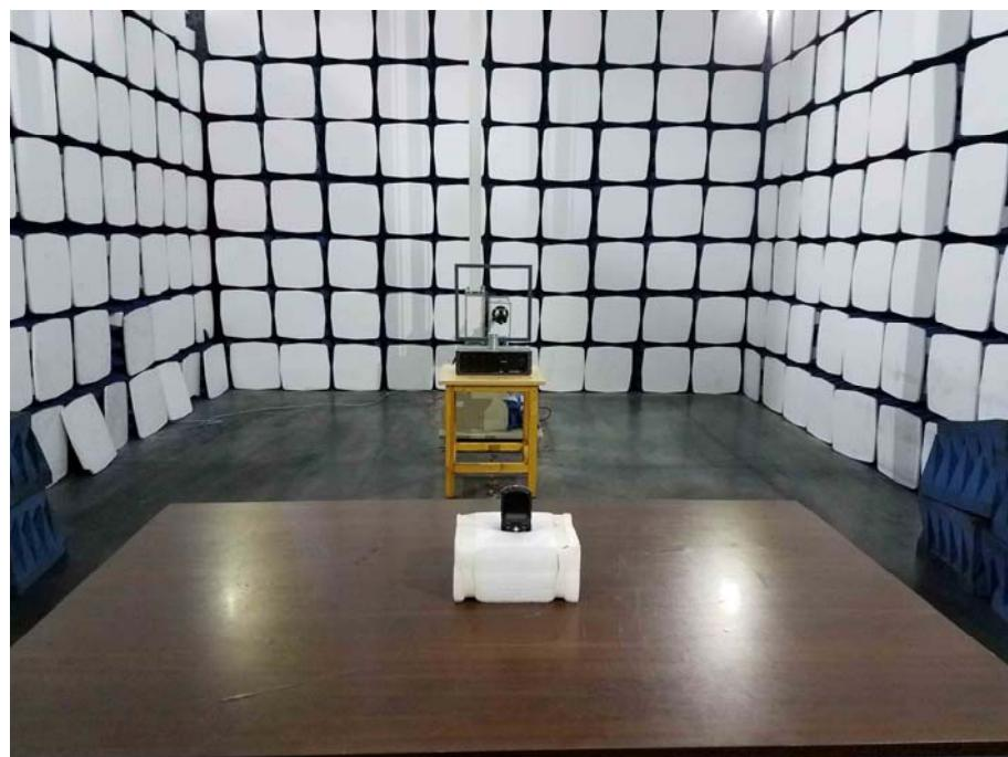
**Radiation Emission Test Setup (30MHz to 1GHz)**
