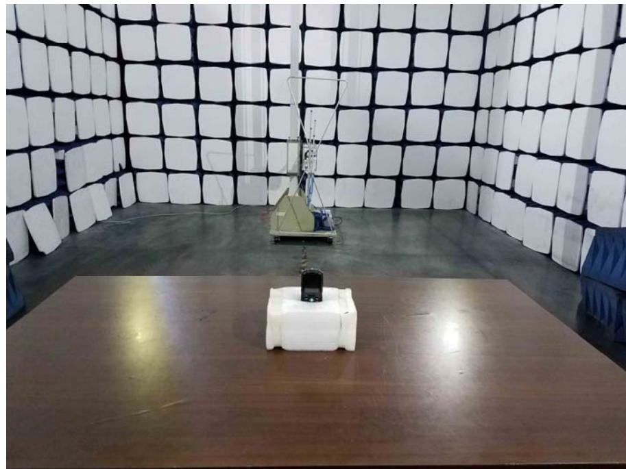
**Radiation Emission Test Setup (Above 1GHz)**
