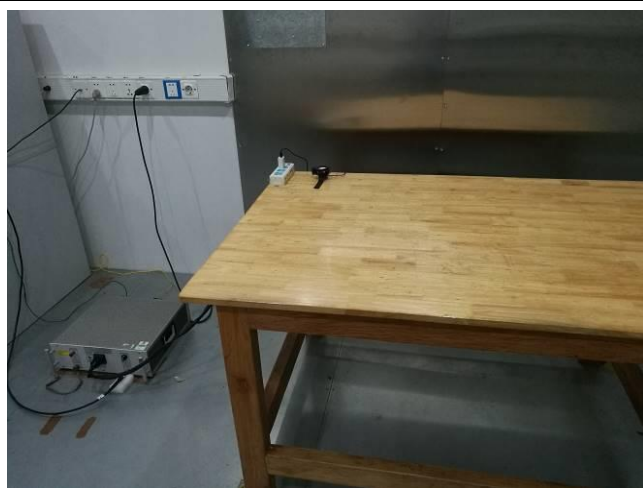
Conducted Emissions Test Setup – Front View
