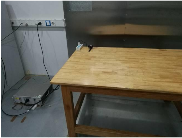
Conducted Emissions Test Setup – Front View
