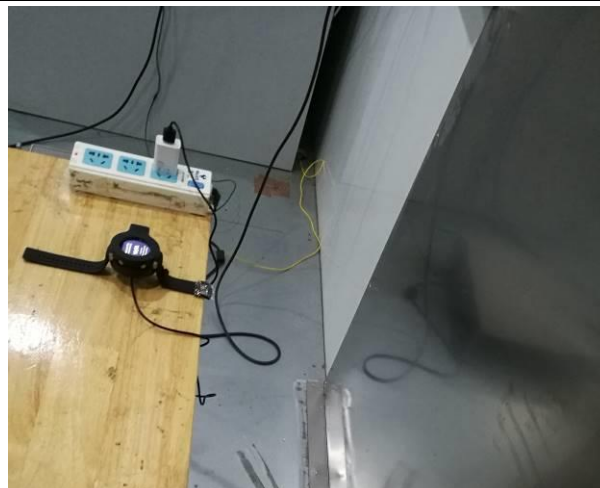
Conducted Emissions Test Setup – Side View
