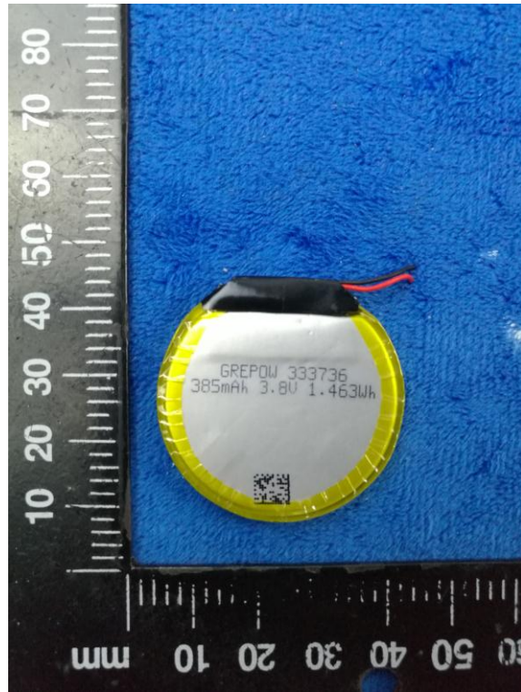
Battery - Front View
