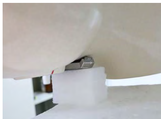
Fig.4 Configuration 2: remove the watchband and make the watch's back touch against the neck phantom area
