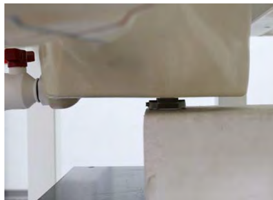
Fig.3 Configuration 1: remove the watchband and make the watch's back touch against the flat phantom
